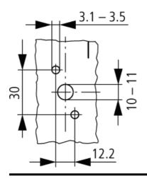
Diameter of drilled hole Door
